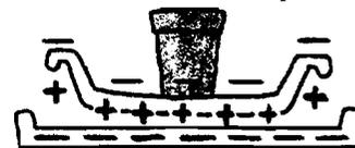
3. When students bring their finger near the rim of the electrophorus, the charge that is not attracted to the cutting board (the negative charge) escapes into their bodies.
