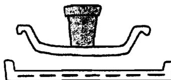
2. When students place the electrophorus on the negatively charged cutting board, the negative and positive charges on the electrophorus separate. Because like charges repel each other, the negative charges on the electrophorus move away from the cutting board, toward the rim of the pie pan. The positive charges on the electrophorus are attracted to the negatively charged cutting board and thus move to the bottom of the pan.
