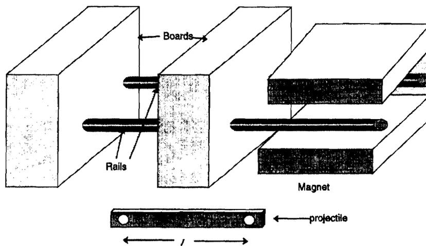
Fig. 1. Projectile with drilled holes and orientation of boards, rails, and magnet for rail gun apparatus.
