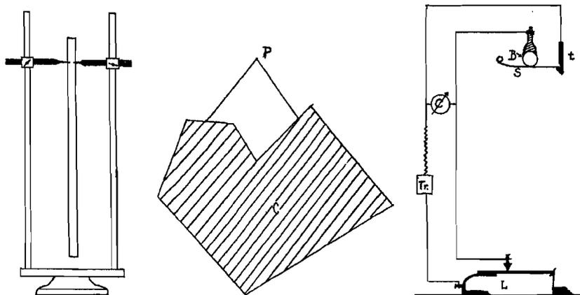
FIG. 1. (Left) Physical pendulum. FIG. 2. (Center) Case where the axis is off the board. FIG. 3. (Right) Falling body apparatus.
