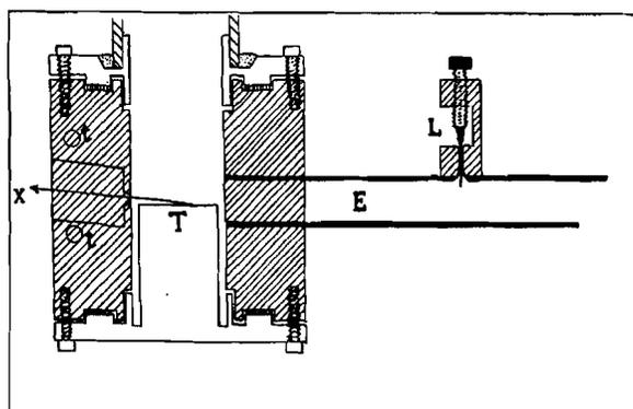
FIG. 1. *E*: exhaustion tube; *T*: target; *t*: watercooling tubes; *L*: leak; *X*: x-rays.
