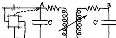
FIG. 5. Arrangement for study of coupled resonating circuits.
